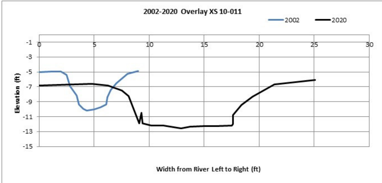
Figure F-6. Change in cross-sections for 10-011 between 2002 and 2020.
